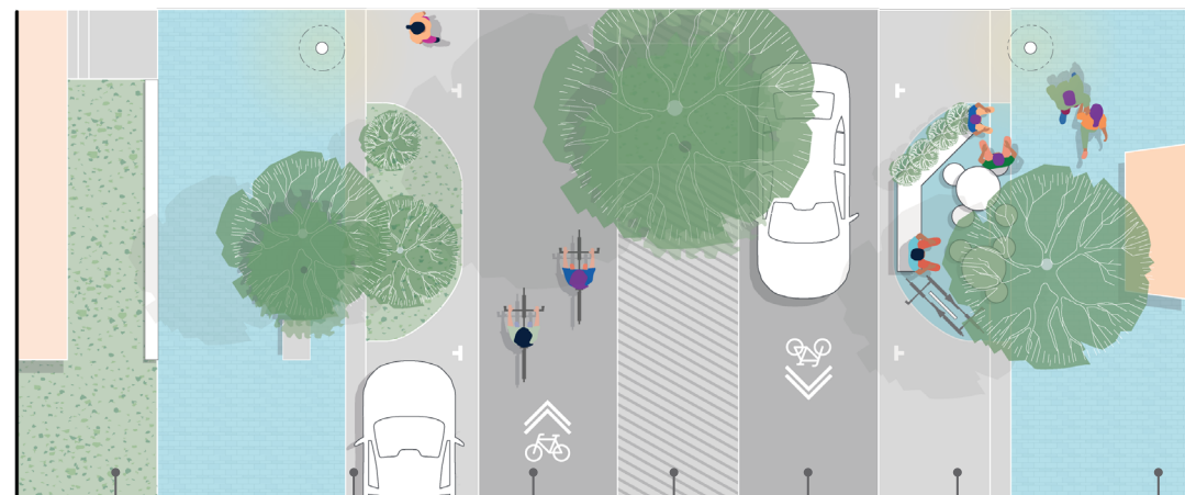
Residential Yard | Rain Gutter | Sharrow | Median | Car Lane | Parking Lane | Footpath
